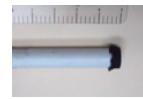
Figure 4. Sensor packaged in plastic tubing with GoreTex cap for casting in fresh paste
