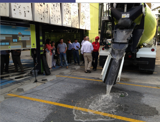
Pervious Pavement Demonstration at the Argos Research Facility
