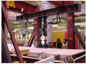
The Minne-ALF can be configured in many different ways to address various test parameters. Load, deflection and other instrumentation data are collected automatically at user-specified intervals. The device is currently being reconfigured to provide direct control over joint widths for tests of joints with misaligned dowels. It can also be used to investigate a wide range of other pavement design, rehabilitation and behavior issues for both concrete and asphalt pavements, including:
