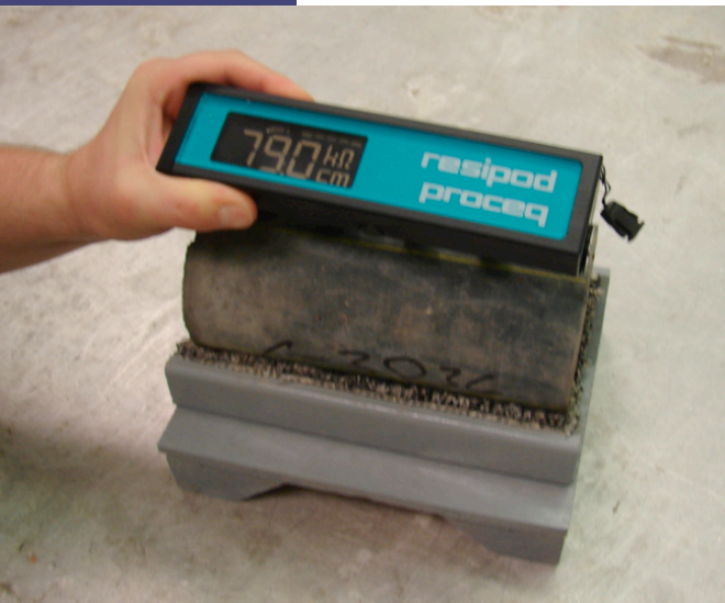
Surface Resistivity Test Being Conducted on a 4" x 8" Cylinder
