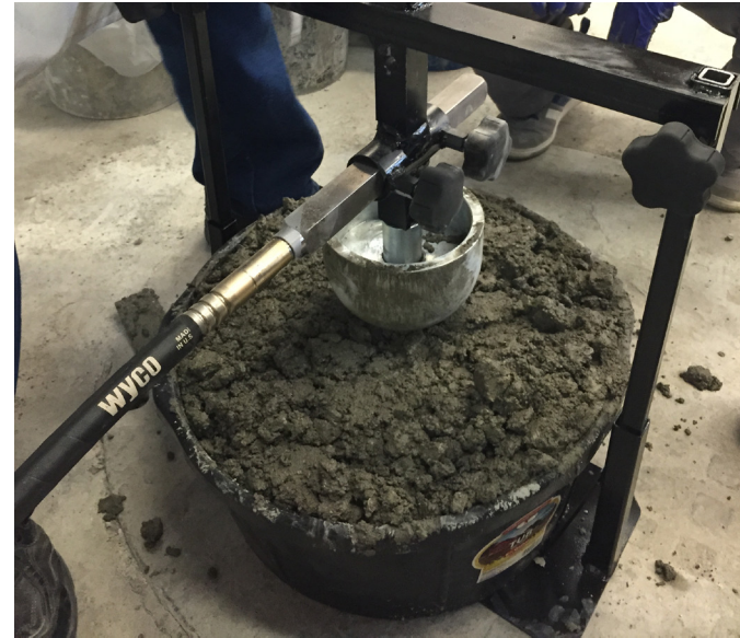
Performance Engineered Mixtures can be assessed using a variety of methods, including V-Kelly Test
