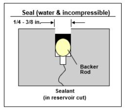
Sealing and filling joints are different treatments. The picture to the left is an example of a sealed joint. This type of joint treatment helps to prevent intrusion of water into the subgrade and also helps keep incompressible materials out of the pavement section. The Backer Rod helps create the seal keeping water out and reduce leaking of sealant material downward. Installation of sealed joints require two sawcuts and they with are relatively wide, as indicated in the picture.
