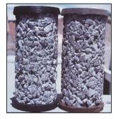
doubles as a pavement and a stone base is a critical component of the system as a reservoir to temporarily hold water. In a pervious concrete mix, shown in the picture to the left, fine aggregates (sand) are typically removed leaving the cement-water paste and a single sized rock with a 10%-15% void space. Water from rainfall readily passes through the concrete surface layer into the stone base reservoir which has a
