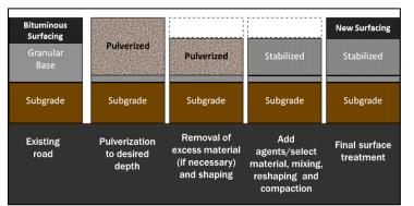
surface and aggregate base, blending the materials into a single matrix. Once this blended material is graded and shaped, it is mixed with cement which stabilizes it and creates a suitable base on which to place a final pavement surface. The dotted rectangles in steps three and four of the picture represent a significant reduction in material removed from the project site when compared to the full depth of bituminous surfacing and granular base shown in step one.
